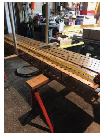
Building a windchest (an air-tight wooden box that holds pressurized air and delivers it to the pipes, which sit on top of it, to produce sound). The board with holes is a toe board. The pipes get installed on top of the toe board (see first photo below) and underneath are valves that control the flow of air to the pipes (see second photo, below).
