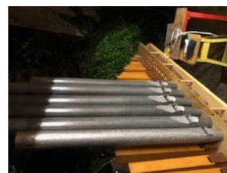
Building a windchest (an air-tight wooden box that holds pressurized air and delivers it to the pipes, which sit on top of it, to produce sound). The board with holes is a toe board. The pipes get installed on top of the toe board (see first photo below) and underneath are valves that control the flow of air to the pipes (see second photo, below).
